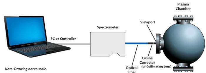
**Figure 1:** A modular spectrometer setup can be configured for plasma measurement in a vacuum chamber.
